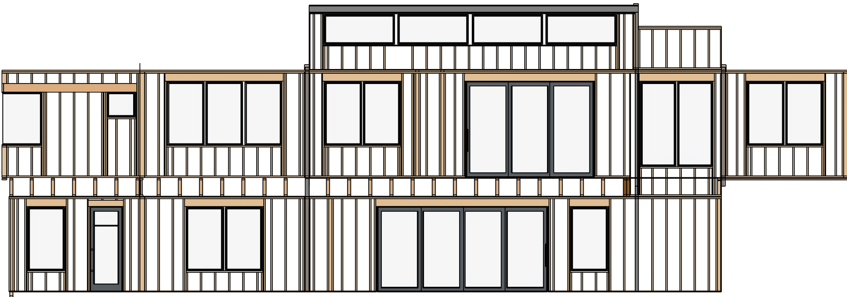
F2 REAR SECTION FRAME DETAIL 3/16"=1'
