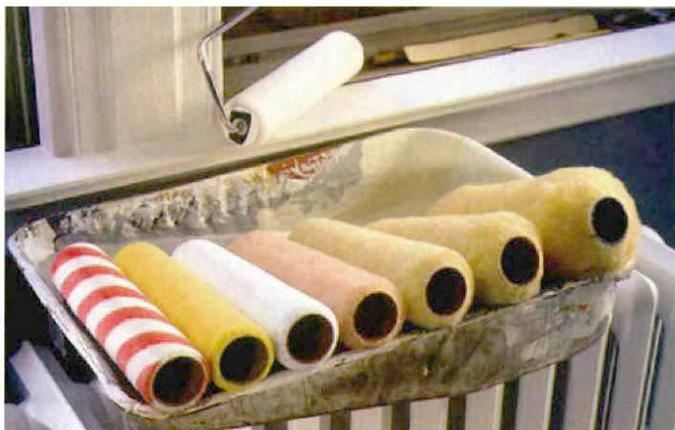
There are several factors I consider when choosing a roller pad (photo above). The first is the surface I'm going to paint. For smooth surfaces, a roller pad with a short nap (1/4 in. to 1/2 in.) is fine. But if you're covering a heavy stucco, you may
