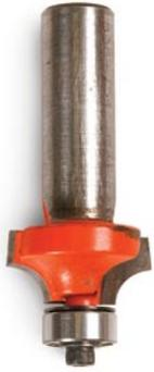
After ripping the beam bottom to width, I mill the edges on a router table with a ¼-in. roundover bit. I make one pass with the bit depth set to mill a simple roundover. I then raise the bit ⅛ in. and flip the stock for a second pass that creates a quirked, or shouldered, edge, which conceals the joint.
