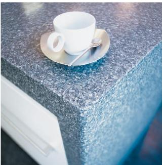
Polished or honed, but always made with aluminum. Alkemi uses only aluminum shavings in its countertops. The variety of colored shavings, like bronze or copper, is acquired by anodizing the shavings prior to mixing them with resin. Alkemi tops are available with either a smooth, honed surface (top) or a textured surface (bottom).
