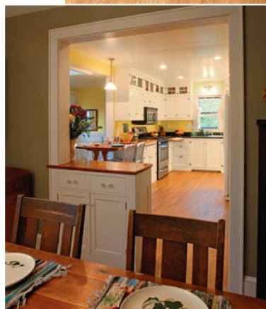
The kitchen/dining connection. Opening up the wall between the kitchen and the dining room extended the views from one to the other. The countertop between the two rooms serves as a buffet for dinner parties. Like the views, the cabinet drawers open into both the kitchen and the dining room. Photos taken at A and B on floor plan.
