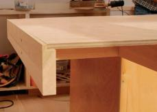
**Edges concealed.** Although the plywood is hidden by the drawers and trim, the author recessed the plywood into the frame and covered the sides with a band of poplar.
