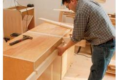
**Check the fit.** Because the frame's strength depends on the locations and the tightness of the bridle joints, dry-fit the entire frame around the cabinets before applying glue.
