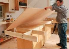
**Add the top.** Once the frame is assembled, measure and cut a piece of ½-in. plywood that will strengthen the base for the solid maple countertop.
