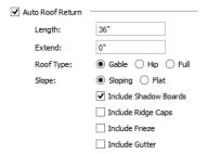
Specify the horizontal **Length** of the returns in inches; the distance to **Extend** the returns past the main roof overhang; the style of roof return; and whether the returns are sloping or flat. As long as your model has a roof, the specified roof returns will be generated when you click **OK**. For more information, see "Roof Returns" on page 531 of the Reference Manual.
