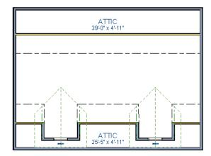
8. Select each of the knee walls and move them back so that they are in alignment with the ceiling plane. When **Object Snaps** are enabled, the walls will snap into position when they are close to the Ceiling Break Lines.
