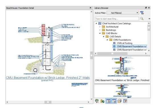
5. Select File> Print> Drawing Sheet Setup and specify a Drawing Scale for the CAD detail in the Drawing Sheet Setup dialog. 2 inches = 1 foot works well in this case.
