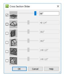
5. Select the horizontal cut line and use the **Position** slider to specify the location of the cutting plane. See "Cross Section Slider" on page 930 of the Reference Manual.
