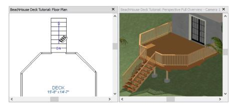
4. In most cases when using the **Click Stairs** stool, an opening will be added automatically to the deck railing at the top of a staircase.
