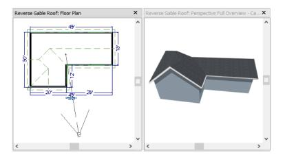
The gable wall on the left produces roof planes that extend too high and interfere with the roof over the front extension of the house. To avoid this, use the Break Wall tool to divide the left wall into two different sections. The upper section can then be specified as a Full Gable without affecting the lower section.
