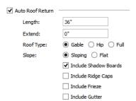
Specify the horizontal **Length** of the returns in inches; the distance to **Extend** the returns past the main roof overhang; the style of roof return; and whether the returns are sloping or flat. As long as your model has a roof, the specified roof returns will be generated when you click **OK**. For more information, see "Roof Returns" on page 529 of the Reference Manual.
