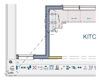
When objects are very close to one another in floor plan view, it may be difficult to select the intended object. When an object is selected, click the Select Next Object edit button or press the Tab key to select a nearby object. See "Select Next Object" on page 187 of the Reference Manual.
