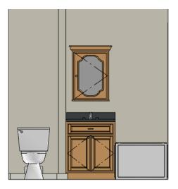
1. On Floor 2, select **3D> Create Orthographic View> Wall Elevation**, then in the Master Bath, click and drag a view towards the cabinet containing the sink.
