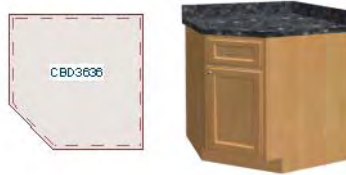
Corner cabinet with diagonal door
