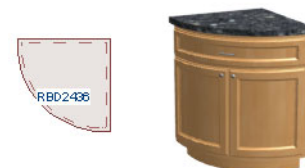
Radius End cabinets have a 90° arch
