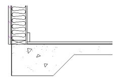
You can also specify the **Chamfer Height** and **Width** before the Slab Footings are created in the **Slab Footing Defaults** dialog. See "Foundation Panel" on page 413.
