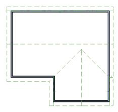
The triangular area of overlap between the main roof and the gable must be defined as a Truss Base.
