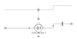
4. Click and drag the edit handle associated with the break parallel to the cutting plane to adjust the position of the step.
