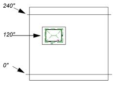
Elevation lines create a terrain grade; an elevation region creates a building pad.
