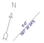
The same line's angle is set to show Bearings, which reference the North Pointer.
