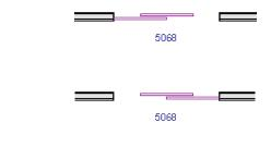
Note: For a Pocket Door to change Opening Side, there must be enough room for the entire door to fit in the wall on that side.
