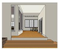
In 3D views, you can adjust the default floor and ceiling height for the entire floor, the floor and ceiling height for an individual room, or the top and bottom heights of an individual wall. See "In 3D Views" on page 433.
