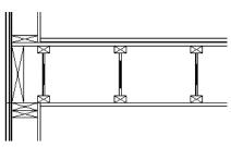
*I-joists, a rim joist, and wall plates cut in a cross section view*
