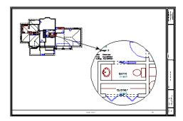
Because the view on the right was sent to layout at a scale other than that of the original, it is subject to layout line scaling.
