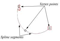
**Connect Electrical** splines cannot be snapped to one another: they can only snap to electrical objects. Once drawn, though, additional vertices can be added and used to form complex curves. See "Editing Spline Based Objects" on page 246.
