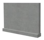
The initial foundation wall type and footing size are specified in the **Foundation Wall Defaults** dialog. These values can be changed for individual walls in the **Wall Specification** dialog. See "Wall Specification Dialog" on page 404.
