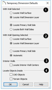
With Wall Selected - Specify how walls are located by temporary dimensions when a wall is selected.
