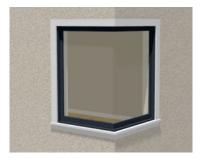
Angled top, or shaped windows can be components of corner windows as long as their heights are equal at the corners. Windows with single or two segment tops can be used, but windows with three cannot. If a two segment window is used, the segment nearest the corner must be flat.
