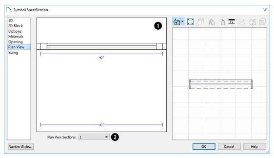
An editable diagram of the symbol's representation in floor plan view displays here. The settings here also affect how many units the symbol contains as well as their size in both 2D and 3D views.
