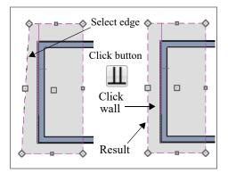
You can also make the selected edge parallel by rotating the entire object. See "Make Parallel/Perpendicular with Polyline Based Objects" on page 271.
