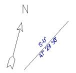
*Line angle shown in degrees. This does not reference the North Pointer.*
