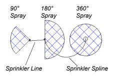
Sprinkler head display in 3D views; however, Sprinkler Lines and Splines do not.
