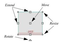
• Click and drag the Move handle to move the object according to the currently
