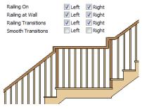
Check Smooth Transitions on Left and/ or Right to specify the placement of smooth connections between stair and landing railings. Not available for ramps.
