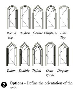
• Check **Reflect** to reflect the arch, top to bottom. This is typically used with windows rather than doors. Not available if a lintel is specified for the selected door. See "Lintel Panel" on page 567.
