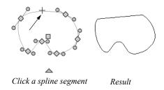
If you reselect the spline, you see that the two control handles point toward the straight section from each vertex point on either end of the straight section.
