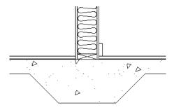
• When the Slab Footing defines the edge of a slab, a thickened slab edge results.
