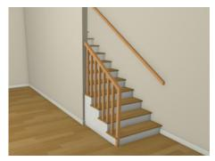
Partial railings can be created by specifying the stairs as winders and increasing the **Max Tread Contraction** in the **Staircase Specification** dialog. See "Style Panel" on page 768.
