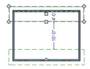
Select both roof planes and check Curved Roof in the Roof Plane Specification dialog. Set the Angle at Ridge to 33.6901°, which is the same as 8 in 12. Notice that the Angle at Eave is almost flat.
