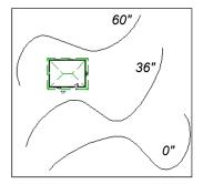
Elevation splines before terrain generation
