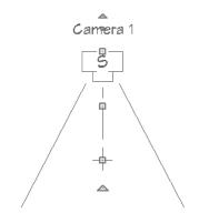
• Camera symbols representing cross section/elevation views indicate the clip plane position, line of sight, and back clip plane position if there is one.
