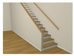
If any balusters extend beyond the railing, eliminate them by unchecking Left Railing or Right Railing in the Staircase Specification dialog. See "Style Panel" on page 768.
