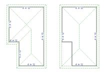
On the left is the baseline polyline as it was originally produced and the roof plan it creates.
