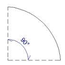
• Arc Length - The length of the arc along the curve.
