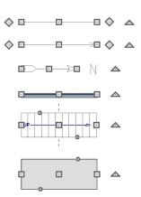
Other objects, such as stairs, foundation walls with footings, and roads, have additional edit handles that allow you to concentrically adjust the object's width.
