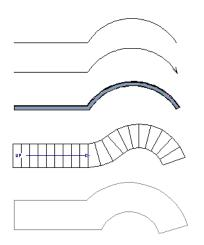
Other objects, such as connected stair and road segments, have additional edit handles that allow you to concentrically adjust the width of all segments of the object. If Connect CAD Segments is disabled, clicking on a CAD polyline edge selects the individual edge rather than the entire polyline. See "Disconnect Edges" on page 220.
