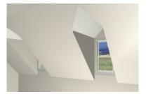
A floating dormer can be placed in plan view on the same floor that its underlying roof plane displays on, or it can be placed on the floor above. Normally, it does not matter what floor the dormer is on; but in some cases, it may need to be on the floor above so that the dormer walls do not interfere with walls or railings in the room below.
