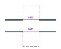
Unlike other door types, the Swing side of a garage door cannot be modified using the edit handles.
