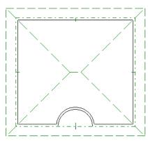
• Spanning the concave curved wall with a straight Baseline and produce a roof plane for it from that.
