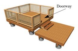
To open a railing across an entire section, resize the doorway's **Width** so that it is greater than the length of the railing in the **Door Specification** dialog. The opening resizes to the maximum width possible for that space. See "General Panel" on page 561.
