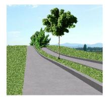
A Cul-de-sac is a road object with a special, rounded shape that can be placed at the end of a Road object. Select Terrain> Road> Cul-de-sac and click on the end of a road to place a cul-de-sac at that location. Culs-de-sac cannot be connected to the edge of Road Polylines.
