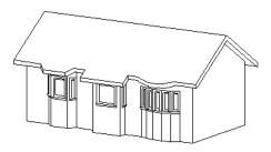
For this roof style, the ceiling heights of the window unit and the adjacent room must be the same. If you lower the ceiling of the window unit and then build the roof, a lower hip roof over the window is created. See "Floors and Ceilings" on page 614.
