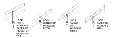
• Specify the **Height** and **Pitch** of the selected roof plane(s). Heights are measured from the top surface of the roof plane(s) rafters or trusses. See "Roof Planes" on page 800.
