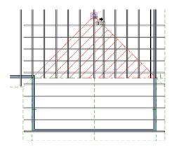
Trusses drawn perpendicular to the baseline of a Truss Base go under the Truss Base. Trusses drawn parallel to the baseline of the Truss Base become valley fill trusses drawn over it.
