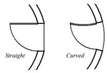
Plinth Blocks - Add an Interior Plinth 8 Block and/or Exterior Plinth Block to the selected door. Plinth blocks do not display in 3D views, but are counted in the Materials List.
