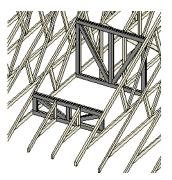
Draw a new truss from an existing truss to the roof edge, as you would to draw a hip or end jack truss; or draw a truss between two trusses, forming a girder. This may be necessary for a large opening, such as a skylight.
