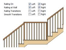
Check **Railing Transitions** on **Left** and/ or **Right** to create "gooseneck" connections between stair and landing railings. This option only has an effect when **Rail Passes Over Newel** is checked. Not available for ramps.
