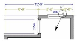
3. Drag it perpendicular to the direction of the arrows, away from any dimension-
