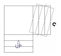
4. The stairs wrap around the corner. Notice that the Up arrow displays on the most recently edited stair section.
