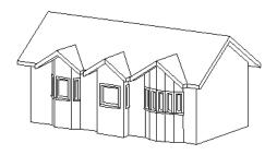
To create a gable roof over a normal window, use the Gable Over Door/ Window edit button. See "Gable/Roof Lines" on page 827.
