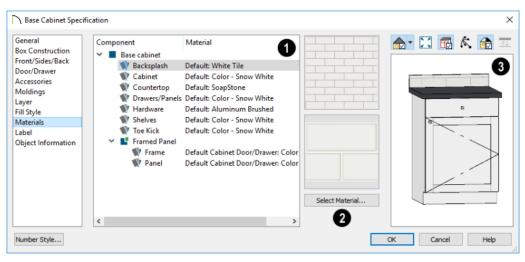
The table on the left side of the panel lists the components of the selected object that can be assigned unique materials, along with the names of those materials and whether or not the default materials are used. Some objects may have only one component while more complex objects may have many. As changes are made to the selected object, components may be added to or removed from this table.
