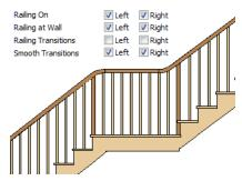
Check both **Railing Transitions** and **Smooth Transitions** to produce a handrail like this:
