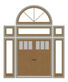
Notice how the windows and door in this example are separate, with spaces between them. Doors and/or windows can also be organized into a unit in which there are no spaces between the windows and door units, and the casing between them is shared. To help organize their display in plan view, you can place stacked windows of varying heights on different Window Levels. See "Window Levels" on page 588.
