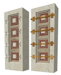
A custom chimney can be designed using 3D Boxes and Cylinders and the Union and Subtract edit tools.
