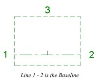
Most roof planes are drawn over a wall, and the Baseline should be located directly above the outer edge of the wall's Main Layer. See "The Main Layer" on page 398.
