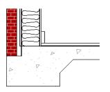
Cross section of monolithic slab brick ledge
