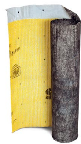
Ready-made rain screen. For an all-in-one rain screen (photo above), plastic mesh ( www.homeslicker.com ) is bonded to the synthetic housewrap Typar ( www.typar.com ). This combination rolls on just like builder's felt (drawing left) for 65¢ per sq. ft. Home Slicker mesh is also available bonded to #15 felt or on its own (no backing). For more on housewrap options, see FHB #177, and online at FineHomebuilding.com .
