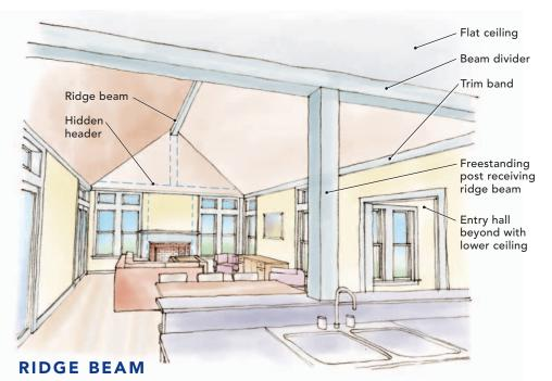
Homeowners often prefer a cathedral ceiling without rafter ties. A sizable ridge beam made of engineered lumber can eliminate the need for rafter ties. Compared to other options, this type of cathedral ceiling may offer the least sense of enclosure, the least density, and the
