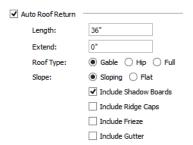
Specify the horizontal **Length** of the returns in inches; the distance to **Extend** the returns past the main roof overhang; the style of roof return; and whether the returns are sloping or flat. As long as your model has a roof, the specified roof returns will be generated when you click **OK**. For more information, see "Roof Returns" on page 523 of the Reference Manual.
