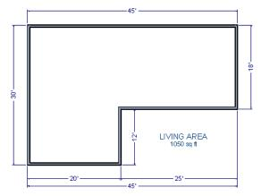
To create a reverse gable in this plan, we need to create three gable walls: two running vertically and one horizontally.
