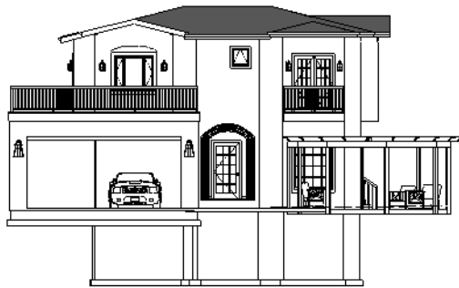
Any Orthographic view can be converted to a CAD Detail. All patterns become lines and colors no longer display. Individual lines can be added and edited.
