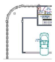
6. Now add two more Elevation Lines i just inside the retaining wall. This helps designate the height of this area when terrain is generated. This elevation line can stay at its default height of 0'0".
