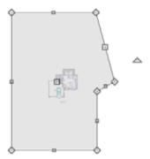
4. Select the bottom edge of the Terrain Perimeter, and click on the **Change Line/Arc** edit button, and notice that this segment changes in to an Arc, which can then be modified using its edit handles. For more information on modifying arcs, see "Editing Arc Based Objects" on page 174 of the Reference Manual.
