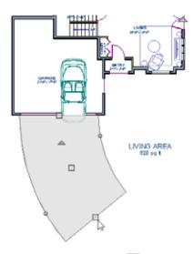
6. Next, add in a Terrain> Road> Straight Road and Terrain> Sidewalk> Straight Sidewalk to complete the design.
